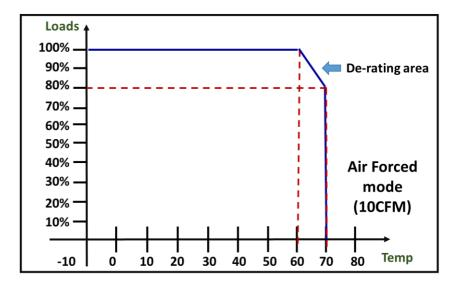
**Note: De-rating Power Output with Temperature**
