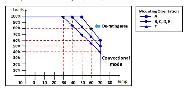
**Note: De-rating Power Output with Temperature**
