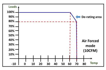
Note: De-rating Power Output with Temperature
